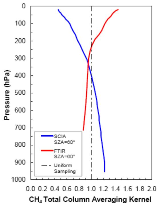
Fig. 1. Total-column averaging kernels for Zugspitze FTIR (red line) and SCIAMACHY-WFMD CH<sub>4</sub> retrievals (blue line) calculated for a solar zenith angle (SZA) of 60°.
