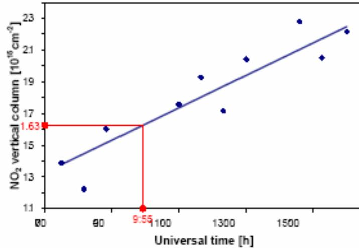
Fig. 4. Zugspitze FTIR NO<sub>2</sub> vertical column data – individual measurements of one arbitrarily chosen day. The blue line is a fit with a constant slope (i.e., the daytime increasing rate of  $1.02 \text{ E}+14 \text{ cm}^{-2}/\text{h}$ ) with only the offset as fit parameter. The red lines illustrate the concept of the “virtual-coincidence column”, here for a 09:55 UT satellite overpass. For details, see text.
