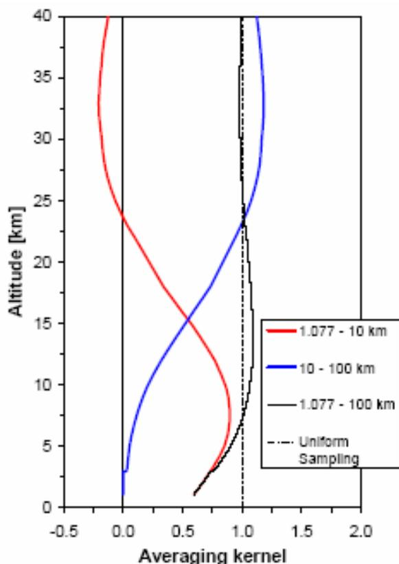
Fig. 12. Averaging kernels for the combined FTIR and SCIAMACHY retrieval of  $\text{NO}_2$ , calculated for a solar zenith angle of  $20^\circ$ . Red curve: Tropospheric partial column averaging kernel (calculated for 1.077–10 km). Blue curve: Stratospheric partial column averaging kernel (calculated for 10–100 km). Black curve: total column averaging kernel for the combined retrieval.
