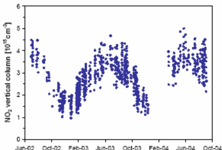
Fig. 2. The Zugspitze FTIR NO<sub>2</sub>-vertical column data set analyzed in this study for SCLAMACHY validation by using as a priori the US 1976 Standard NO<sub>2</sub> VMR profile with the tropospheric part (<10 km) set to zero. Plotted are columns retrieved from individual measurements (10-min integration time).
