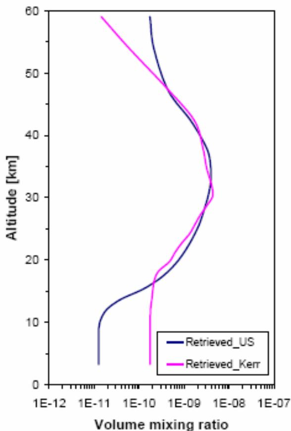
Fig. 1. NO<sub>2</sub> FTIR (profile scaling) retrieval results from one arbitrarily chosen measured Zugspitze FTIR spectrum with SZA=61° using two different NO<sub>2</sub> a priori VMR profiles, i.e., the 1976 US Standard atmosphere (blue) versus the retrieval based upon the standard profile by “Kerr et al.” (Rinsland, personal communication, 1999), distributed with the “refmod99” data set (magenta).
