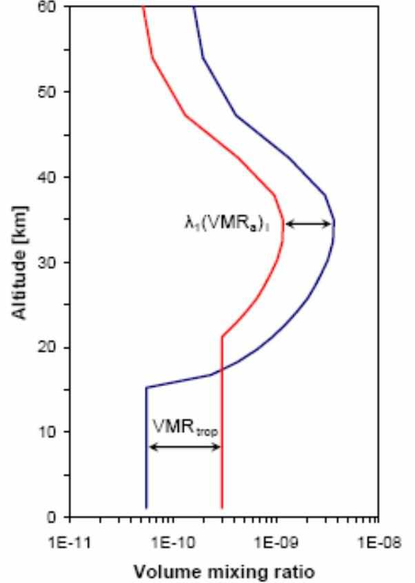
Fig. 10. Schematics for the combined  $NO_2$  retrieval from Zugspitze FTIR and SCIAMACHY using two fitting parameters. First parameter is a scaling factor  $\lambda_1$  applied to  $(VMR_a)_i$ , i.e., the US Standard  $NO_2$  a priori profile (with the tropospheric part set to zero). Second fit parameter is the tropospheric volume mixing ratio  $VMR_{trop}$  assumed to be constant with altitude. Note that the crossing point between both parts of the profile is variable in VMR and altitude.
