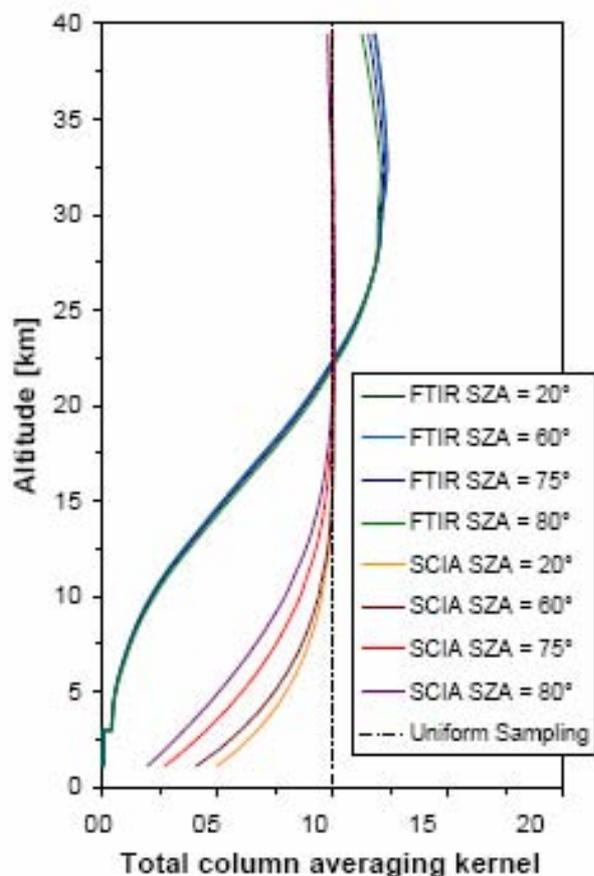
Fig. 8. Total column averaging kernels for Zugspitze FTIR (blue to green lines) and SCIAMACHY UB1.5 NO<sub>2</sub> retrievals (pink to orange lines) calculated for solar zenith angles (SZA) between 20° and 80°. Both FTIR and satellite retrievals are based upon the US 1976 Standard NO<sub>2</sub> VMR a priori profile with the tropospheric part set to zero up to 10 km altitude.
