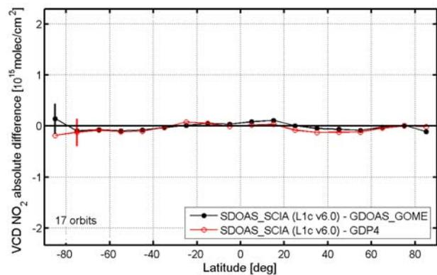
**Figure 2** – Absolute difference between SDOAS and GDOAS NO<sub>2</sub> columns (black plain circles), and between SDOAS and GDP 4 NO<sub>2</sub> columns (red open circles), as a function of latitude.
