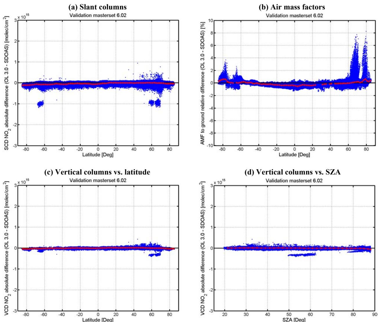
**Figure 3** – Comparison of SGP 3.0 and SDOAS NO<sub>2</sub> retrievals for the SCIAMACHY Master Set: (a,b) slant columns and air mass factors, respectively, both as a function of latitude; (c,d) vertical columns as a function of latitude and of solar zenith angle, respectively. Blue dots refer to individual SCIAMACHY pixels, while red dots show values averaged in 1°-bins.
