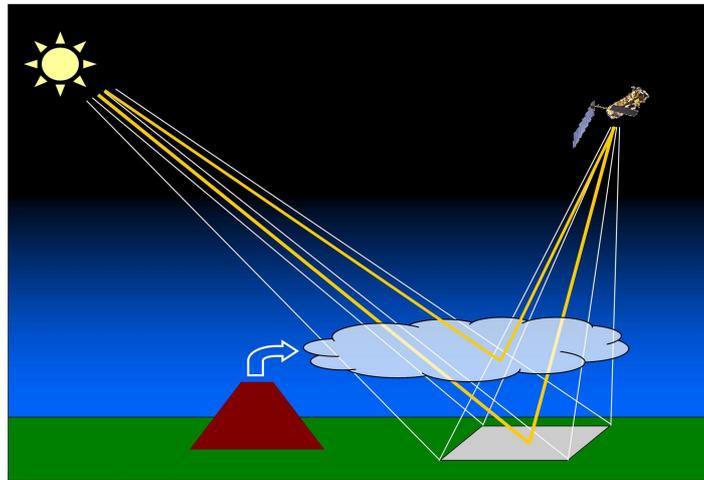
**Figure 1: Sketch of a nadir-viewing satellite UV-visible measurement.**
