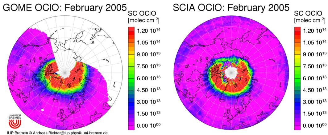
**Fig. 1:** Comparison of GOME (left) and SCIAMACHY OCIO slant columns for February 2005. As result of the permanent failure of the tape recorder on ERS-2, only partial coverage is available from GOME. Similarly, SCIAMACHY measurements have less coverage owing to the alternating limb nadir measurements. Note that the solar zenith angle at overpass is different for the two instruments, resulting in different OCIO photochemistry.
