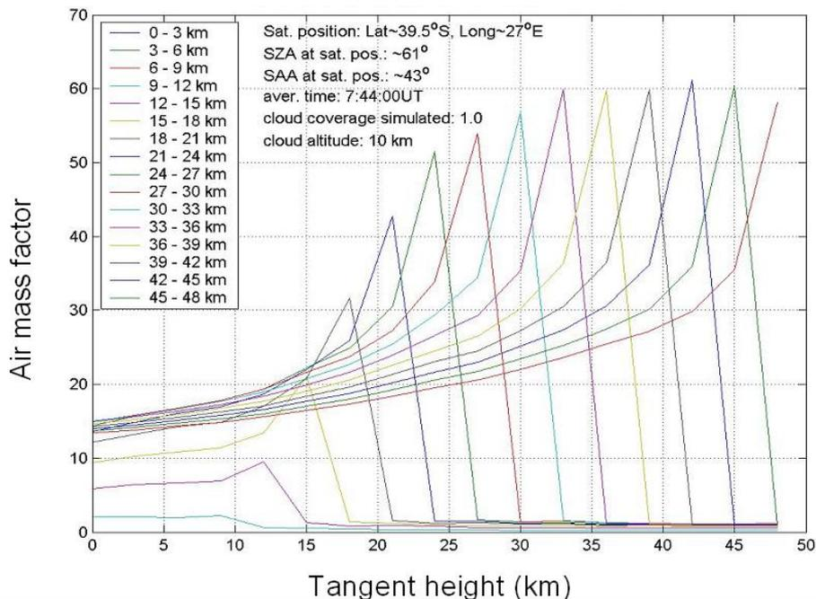
**Figure 4:** Air mass factors for 3 km boxes with constant concentration, as modelled with the RTM TRACY (von Friedeburg., 2003). The air mass factor (AMF) describes the sensitivity of a given observation with respect to the atmospheric vertical column density (VCD). The accurate values of the AMFs depend critically on wavelength, aerosol profile, solar zenith angle and further quantities.
