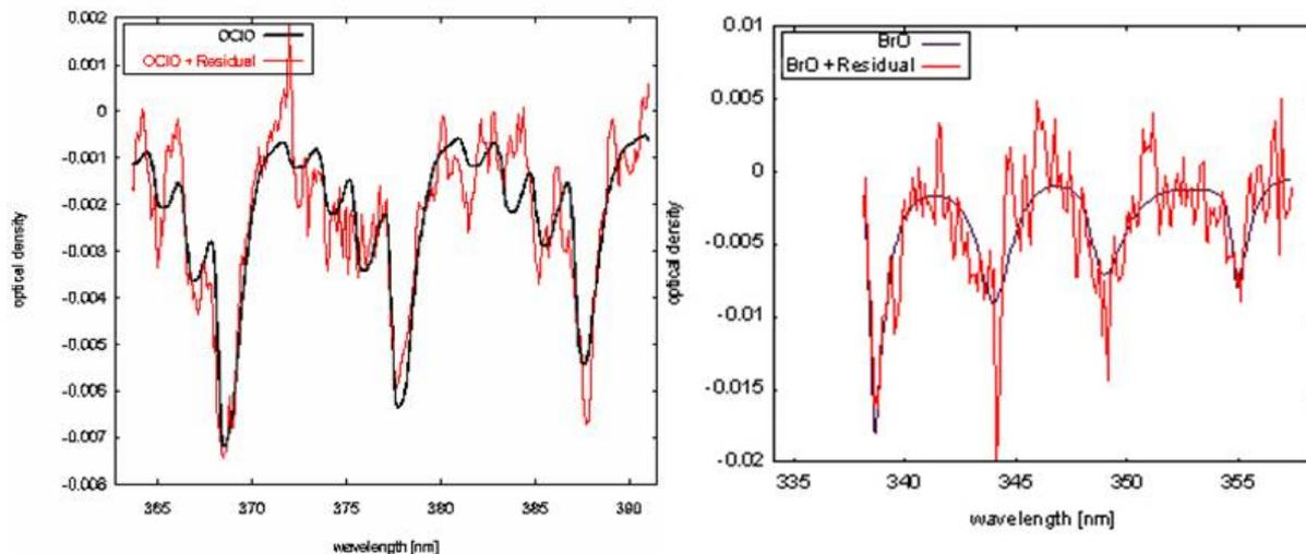
**Figure 3:** Example for an analysis of SCIAMACHY limb spectra for OCIO (right panel) and for BrO (left panel).
