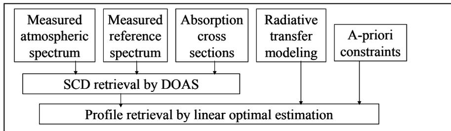
**Figure 2:** Diagram of the HEIDOSCILI algorithm.
